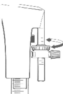
For calibrating purposes turn the screw of the fine adjustment. Turn downwards to increase the volume, turn upwards to decrease the volume.
