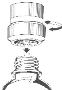
Screw dispenser direct onto containers with thread GL 32 or use adapters to fix on any other threads or ground joint necks. Check the correct fitting. The dispenser can be turned on the flask and fixed in any direction by using the built-in FIX adapter.
