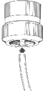
Before using the dispenser please check the dispenser for any damages or glass breakage. Push intake tube over the hose connection of the PTFE valve block.
